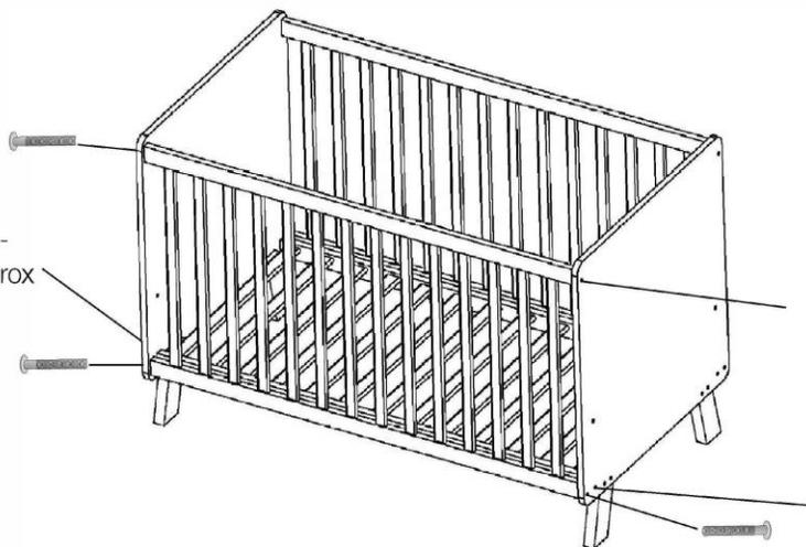
Loosen base connecting bolts approx 3 mm
